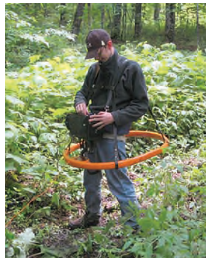
Joshua Shue sets the frequency on the horizontal loop transmitter during an electromagnetic survey near Taylor Mine. Students used electromagnetic techniques to detect and map the location of conductive slates.
