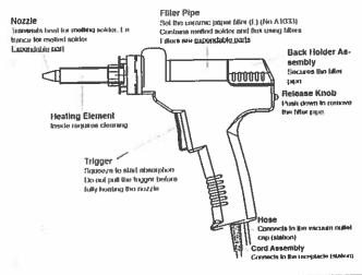
A WARNING: Since the desoldering gun can reach a very high temperature, please work carefully.
